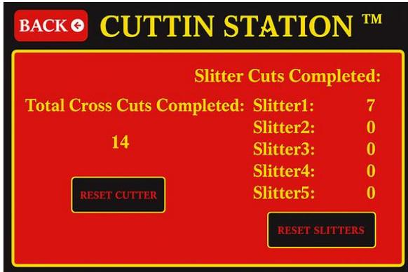
This screen shows the total number of cuts completed during operation
